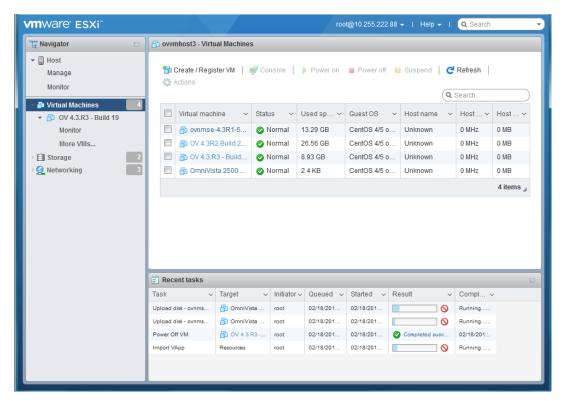
**10.** When the installation is complete (indicated by all three files showing "Completed Successfully" in the Result column of the Recent tasks table), click on **Virtual Machines** in the Navigator Tree on the left side of the screen to display a list of VMs. Select the VM you just deployed. Basic details for the VM are displayed, as shown below.
