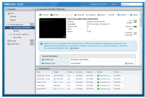
**11.** Click on **Console** at the top of the screen to open a Console and go to <u>Completing the OmniVista Installation</u> to complete the installation.
